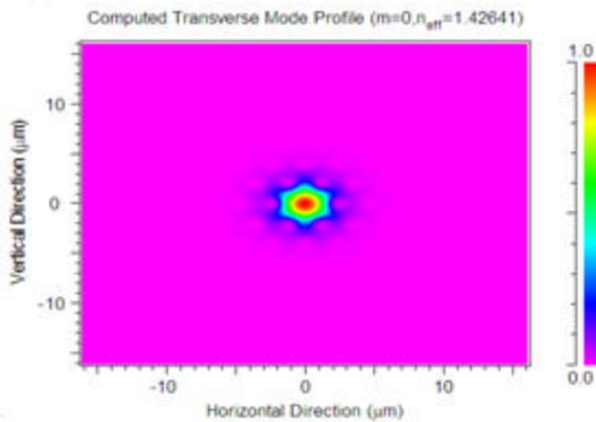
Fig 2: Mode Profile of 2D XY array with a hexagonal cross-sectional pattern of air holes in a silicon fiber.
