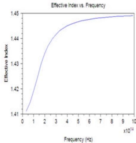
Fig 4: Effective index vs. Frequency graph
