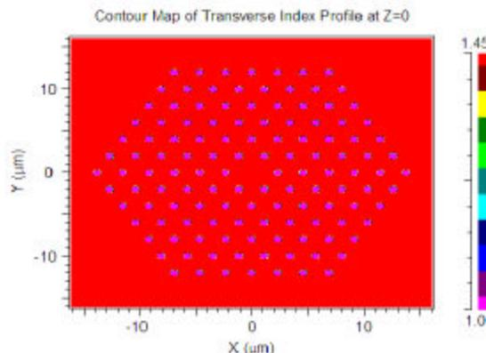
Fig 1: The index profile of 2D XY array hexagonal cross-sectional pattern of air holes in a silicon fiber.
